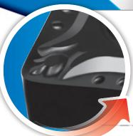
Wiper is assembled by three curves to form a circular arc edge. The nose of wiper provides less profile height on the surface that is formed by the cutting edge, resulting in a smooth turning surface.
